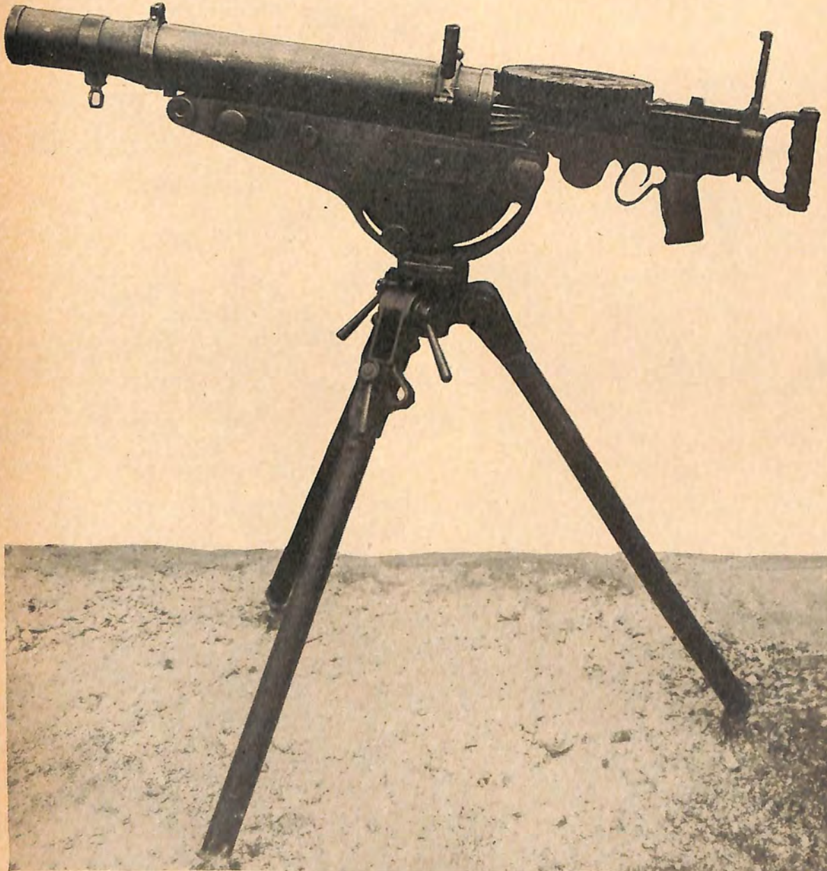
Figure 181. Model 92 (1932) 7.7-mm Lewis type machine gun.
